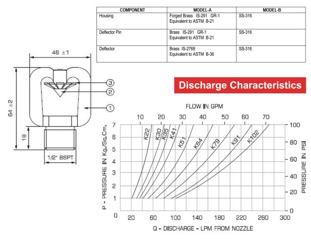
Q = K $\sqrt{P}$ , where P is supply pressure in Kg./sq.cm., K-is nozzle constant in Metric US K Factor = Metric K Factor  $\div$  14.2745
